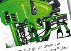
Modern side guard design in combination with the new Safari wheel lock for improved safety.
